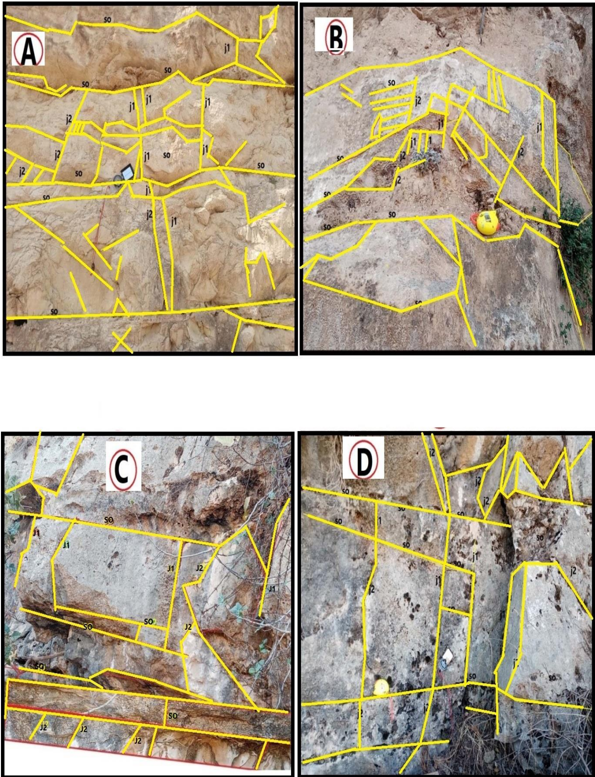
Plate 1: Pictures of the rock blocks located on the right bank of the dam, where (A) represents the spillway station, and (B) is the first station (SR1), and (C) is the second station (SR2), and (D) is the third station (SR3).
